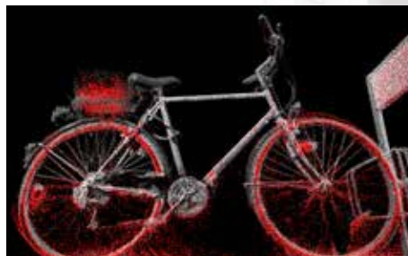
automatic selection of „invalid“ points using the pulse shape deviation attribute information
